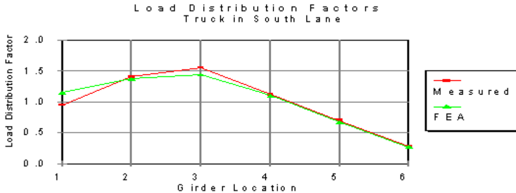
Figure 2.2 Load sharing for the Salmon River Bridge.
